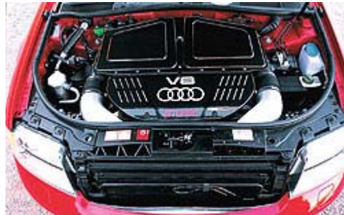
A deliciously smooth 450-bhp twin-turbocharged V-8 and 8-piston calipers with floating rotors are just a few of the treats in the RS 6's plentiful bag of technological tricks.
