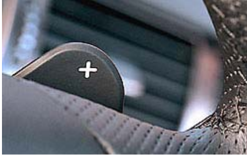
Small paddles on the back of the steering wheel make for quick and convenient shifting of the RS 6's 5-speed Tiptronic transmission.
