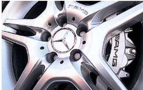
Football-sized 8-piston brake calipers put the bite on massive cross-drilled rotors to help counter the accelerative effects of the supercharged V-8's prodigious power.
