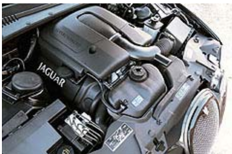
Underhood, Jaguar's 4-cam 4.2-liter V-8 is joined by our test group's only 6-speed automatic transmission to make short work of passing maneuvers and backroads alike.
